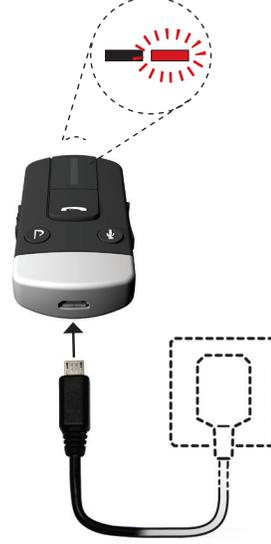
3. Charging is complete when the red LED indicator at the top of the Phone Clip+ turns green with a red blink every 2 seconds. When charging for the first time, the Phone Clip+ should be charged for at least 3 hours, even if the LED turns green before 3 hours have elapsed.
